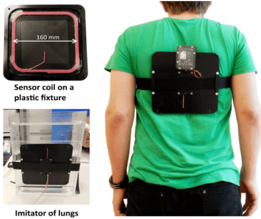
Fig. 4. Photos of the sensor coil on a plastic form, its placement on the imitator of lungs, and at the back of thorax of a volunteer.
