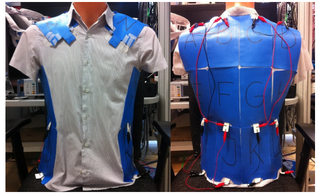
Fig. 2. Picture of the electrode shirt.
