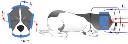
Figure 1. Experimental setup for canine head imaging using four carbon-hydrogel electrodes.
